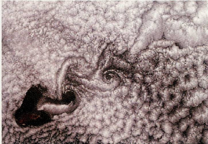
Fig. 9.2 Karman vortex streets in (a) the laboratory, for water flowing past a cylinder [From M. Van Dyke, An Album of Fluid Motion , Parabolic Press, Stanford, Calif. (1982) p. 56.], and (b) in the atmosphere, for a cumulus-topped boundary layer flowing past an island [NASA MODIS imagery].
