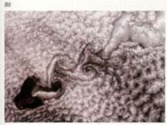
Fig. 9.2 Karman vortex streets in (a) the laboratory, for water flowing past a cylinder [From M. Van Dyke, An Album of Fluid Motion , Parabolic Press, Stanford, Calif. (1982) p. 56.], and (b) in the atmosphere, for a cumulus-topped boundary layer flowing past an island [NASA MODIS imagery].
